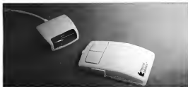
The Cordless Mouse from Practical Solutions: infrared technology is what lets the mouse go "tail-less."
