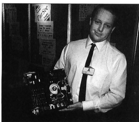
Similar to Atari's own ATW, the ParSec adds another micro-processor for sheer number-crunching power, while retaining an ST as the front-end. Ian Maw, technical director of Elmtch Research, Ltd., is shown holding a prototype ParSec board.
