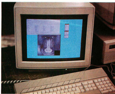
The ATW features a graphical interface not unlike the ST's, but each window has its own dynamic color map and its own palette.
