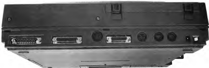
STACY has all of the ports you've become used to on the ST. From left to right across the back are the serial, parallel, external floppy disk drive, DMA, external monitor, MIDI ports and the external power source socket with the reset button adjacent to it.
