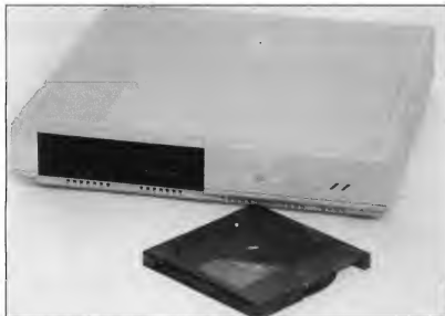
Atari introduced their Megafloppy 44 at Spring COMDEX in Chicago. This new hard drive has a removable cartridge to multiply hard-disk capacity.
