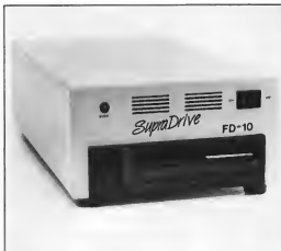
Supra's FD-10 works quite well with Spectre 128—and you don't have to devote a hard disk partition to Mac programs and files. Use the Spectre 128 hard disk formatting function with SCSI device #4.
