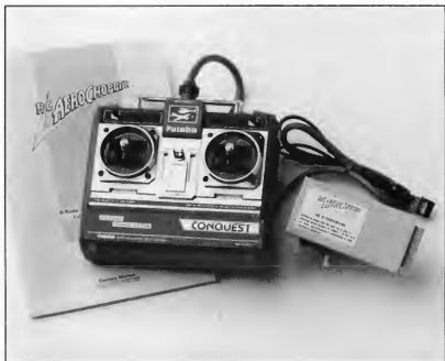
Figure 1: Aerochopper is a unique combination of hardware and ROM-based software that lets you experience the feel of R/C modeling at your ST. The "transmitter" is an authentic Futaba Conquest shell that plugs into a cartridge.
