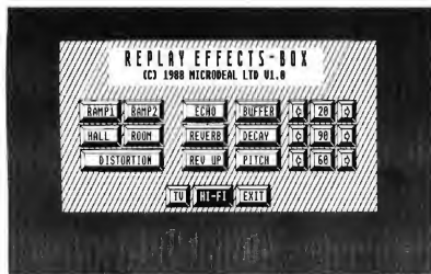
Audio effect selections available with the EFFECTS auxiliary program. This demo program utilizes the Replay 4 cartridge/software to simulate some types of audio signal processing: echo, reverb and distortion.
