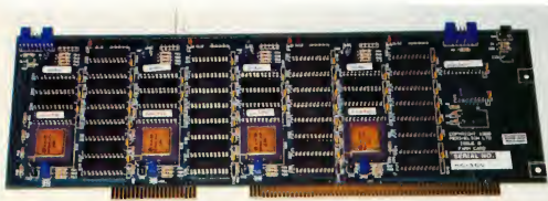
The four gold-colored chips on this ATW add-in card are Inmos T800 transputers. Each card will nearly quintuple the ATW's processing power at a price of only $4,000-$5,000 per card. Naw if there were any software. . .
