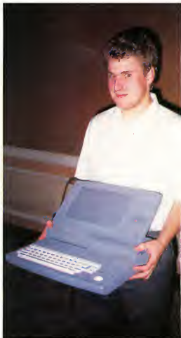
Daryl May is shown holding the foam mock-up of the ST Laptop at the Fall COMDEX Developer's Party. The keyboard in the mock-up is a standard ST keyboard with the keypad, function and cursor keys redesigned and reduced in size.
