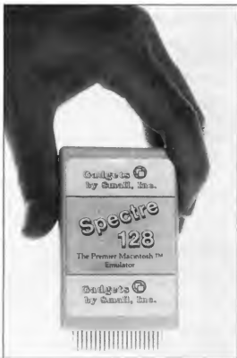
The slender Spectre cartridge shell is the same as the one used in Deskart. You can leave it plugged in all the time, since it is active only when you run the Spectre software.
