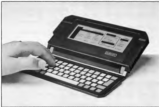
DIP prototype of the Pocket PC, which is currently being "Atari-ized." The only things missing are function keys and a numeric keypad.
