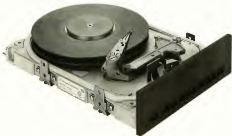
This Seagate 225 is a very typical hard disk. The ST's operating system and hardware must translate your request to open a file into electrical signals that properly position the read/write heads on the platters.
