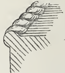
No. 26.—Cable Moulding.
