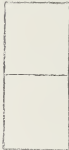
No. 70.—Back of Slab divided into two Panels by a Horizontal Straight Line, as at—
