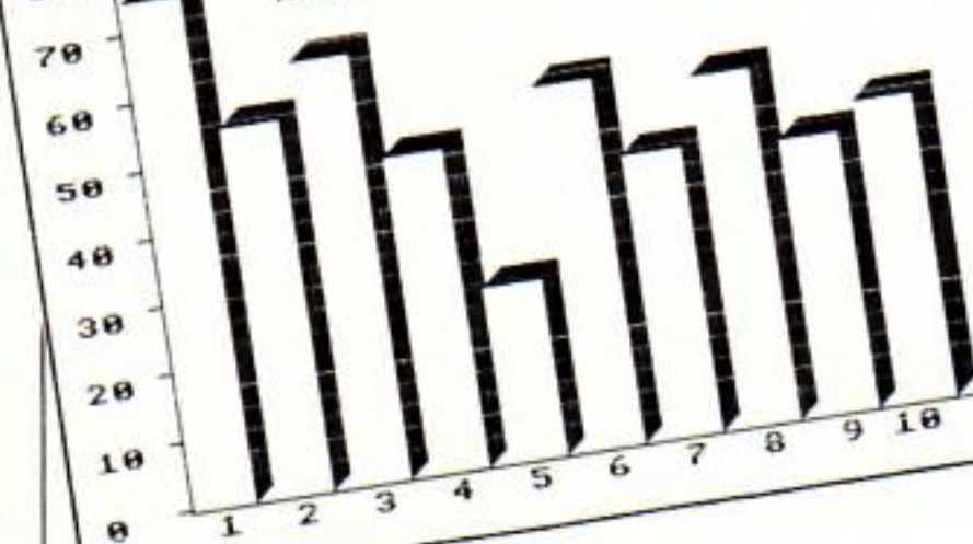
A Histogram To Show The Frequency Of Occurrence OF The Numbers 1-10 When RND(10) Is Used 500 Times
