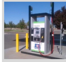
Figure 4. CNG fueling dispenser at public station in Nampa, Idaho (Republic). U.S. Department of Energy
