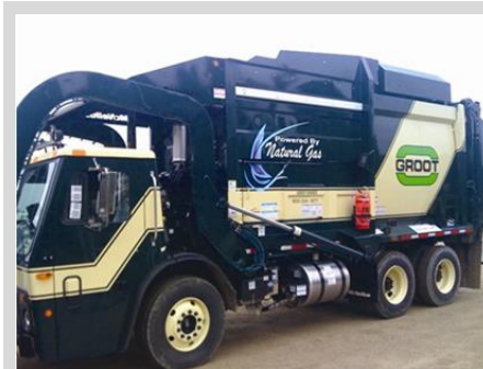
Figure 2. CNG refuse hauler in service with Groot . Chicago Area Clean Cities Coalition
