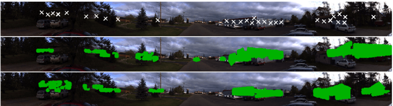
(b) Panoramic photograph and extracted 2D features (top), building points projected onto the image using the RANSAC camera pose (middle) and building points projected using our camera pose (bottom).
