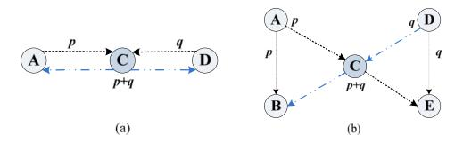
Figure1. examples of information transmission with network coding. Graph (a) is a simple chain topology, and graph (b) is a classic *X* topology.
