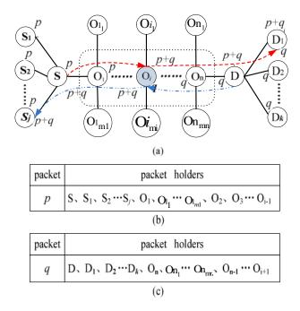
Figure 3. An enhanced coding case. Graph (a) is a basic network model. The information that is appended on packet p is described in table (b), includes all node IDs that which nodes can overhear the packet before it arriving the current node. The information that is appended on packet q is described in table (c).
