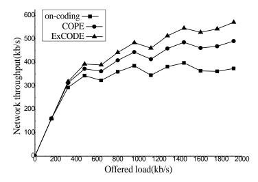
Figure 4. Network throughput vs. offered load
