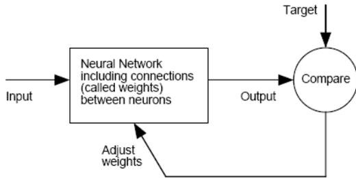
Fig. 1. A schematic of an artificial neural network [2]
