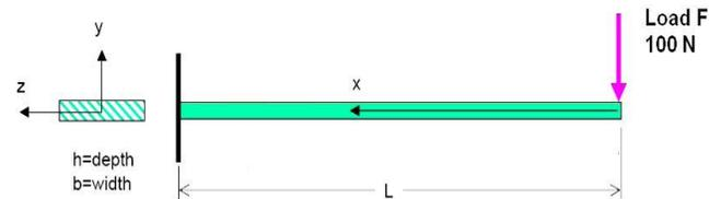
Fig. 4 Cantilever beam with tip loading
